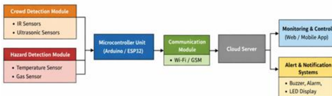
Figure 1. Enhanced Intelligent Crowd Control and Hazard Prevention System for Religious Places Using IoT
