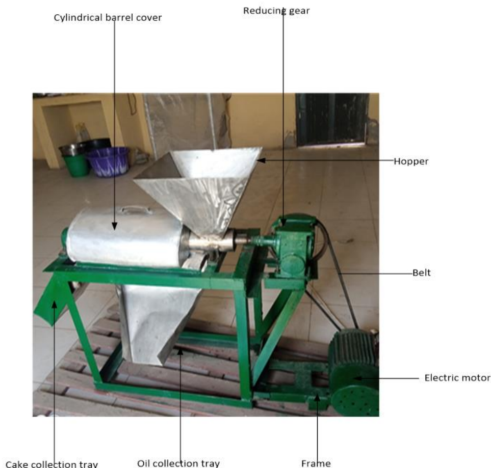
Figure 1. Extruder used for oil expression
