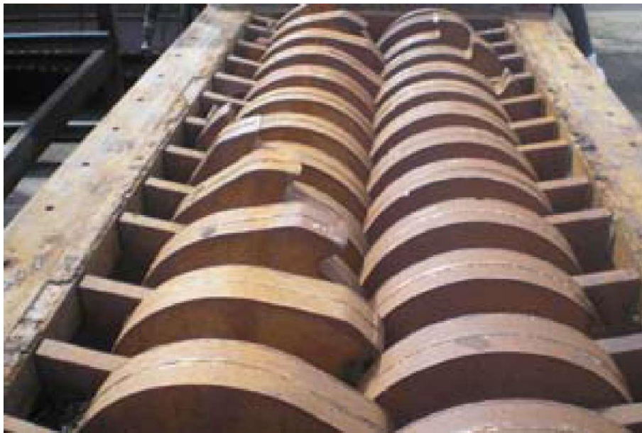
Figure 4. LSHT shredder cutting shaft [SSI 3600 H].
