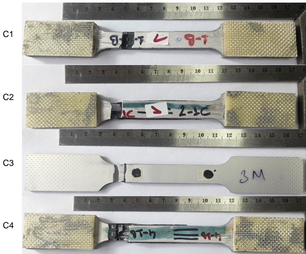
Figure 11. Macroscopic damage observed on carall specimens after tensile testing
