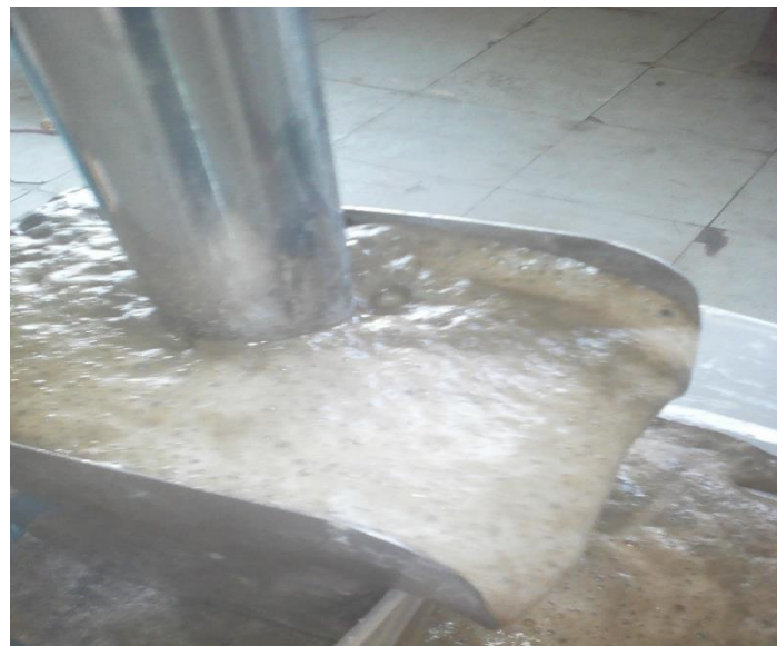
Figure 3. Recovery of gold ore by a standard flotation Cell
