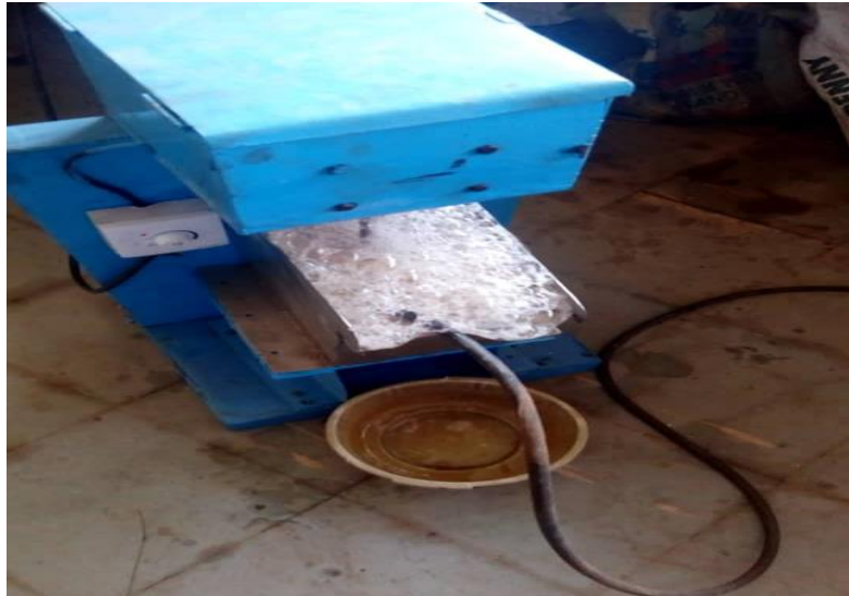
Figure 2. Recovery of gold using Fabricated flotation machine after Aeration
