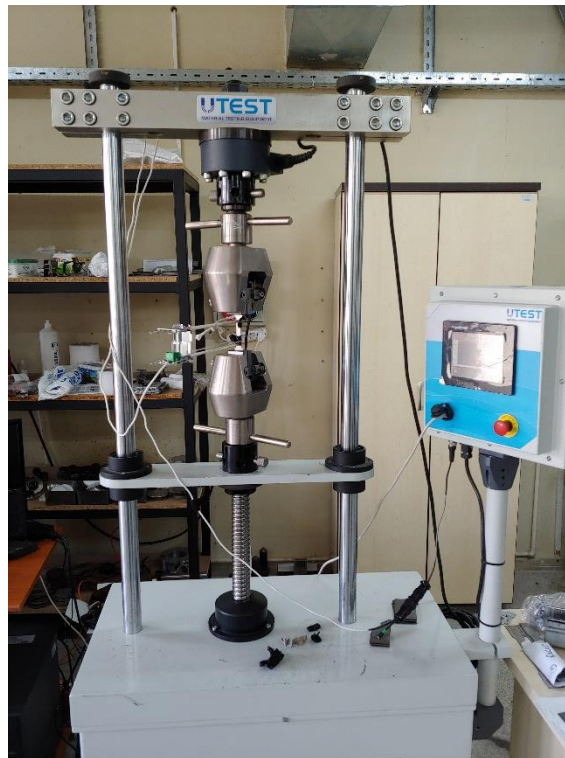
Figure 2. UTEST tensile testing device used in the experiments
