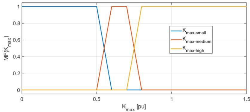
Figure 2. Membership functions for loading rate
