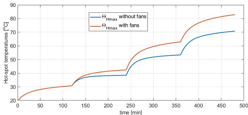
Figure 8. Hot-spot temperatures in cases with and without fan
