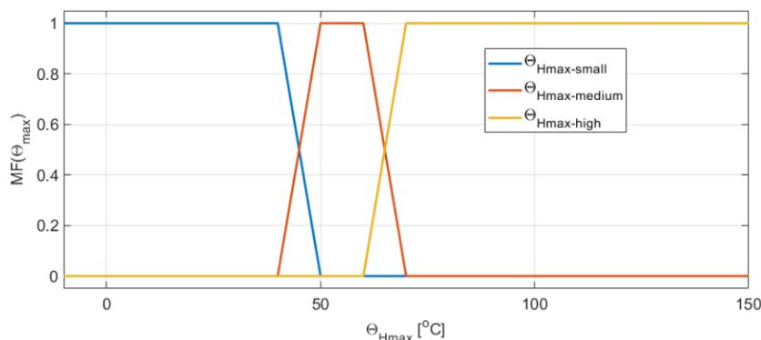
Figure 1. Membership functions for hot-spot temperature
