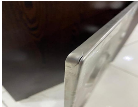
Figure 4. 304 quality INOX cooker panel press printing result form images
