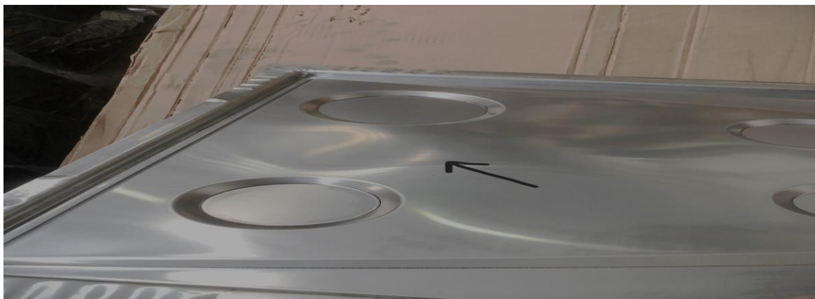
Figure 3. Form image of DC04 7114 quality DKP sheet material as a result of press printing
