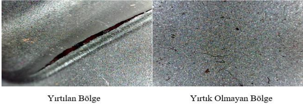
Figure 16 DC04 7114 DKP sheet sample microstructure images
