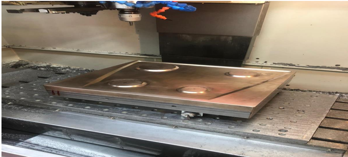
Figure 5. Connecting the male mold to the CNC lathe in the machining center
